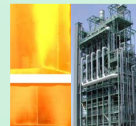
Left: Combustion in an ammonia burner Right: A naphtha cracking furnace
